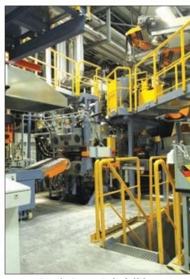
Quintuplex Extrusion Head embedded into locally manufactured downstream
